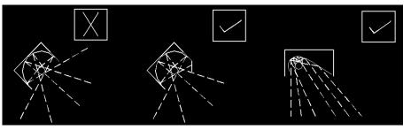
will also be beneficial to use as high a mounting height as possible, giving due regard to the daytime appearance of the installation. The requirements to control glare for the safety of road users are given in Table 2.
