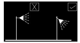
Use specifically designed lighting equipment that minimises the upward spread of light near to and above the horizontal. Care should be taken when selecting luminaires to ensure that appropriate units are chosen and that their location will reduce spill light and glare to a minimum. Remember that lamp light output in LUMENS is not the same as lamp wattage and that it is the former that is important in combating the problems of obtrusive light
